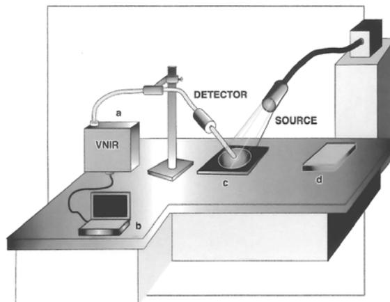
Figure 7. Optical instrumentation used to measure reflectance spectra of macroalgal and toxic phytoplankton HABS in Lee County coastal waters.
