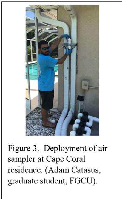
Figure 3. Deployment of air sampler at Cape Coral residence. (Adam Catusus, graduate student, FGCU).
