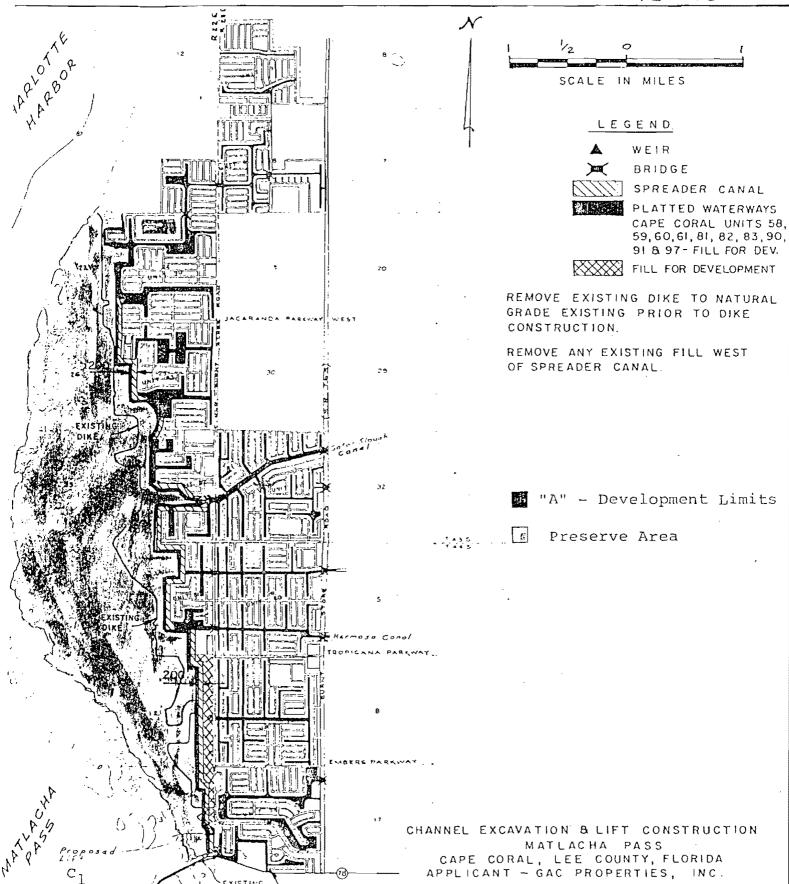
REMOVE PLUG AND SLOPE BANKS TO OBTAIN UNIT 58 PLAT DIMENSIONS
